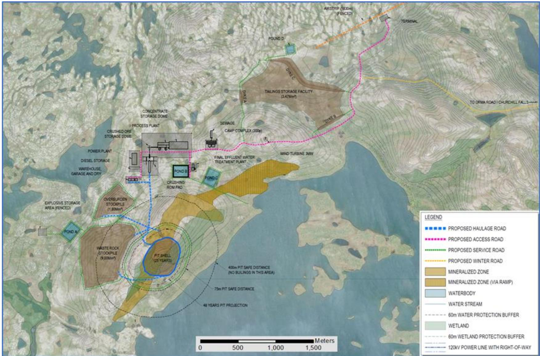
**Figure 2 – Conceptual Layout of Open-Pit Operation Infrastructure, Crater Lake, Scandium + REE TG Zone**
