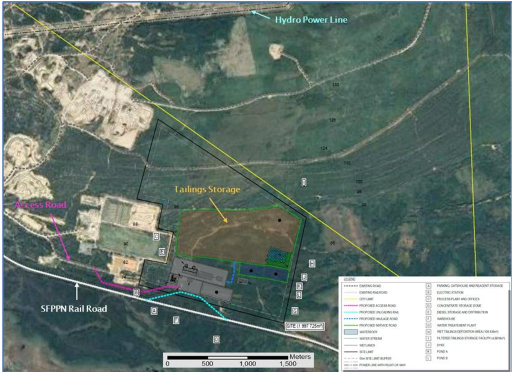
Figure 3 - Conceptual Layout of Process Plant and Tailings Site Infrastructure, Sept-Iles, QC
